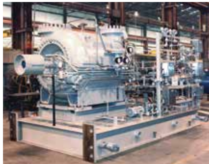
Bolt-up base to gas turbine drive, offshore platform, Malaysia
