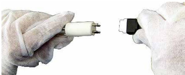
FIGURE 63 - INSTALLING V-RAY AND V-MAX GRID LAMPS
