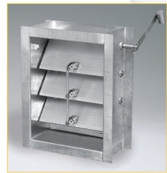
CBS 92 — Extruded Aluminum Blades in 229x51mm Galvanized Steel Frame to meet extra heavy duty conditions. Max. system velocity – 4000FPM Max. air leakage – 0.45% with seals and 2.5% without seals Min. size – 152x152mm Max. size – 1524x2438mm
