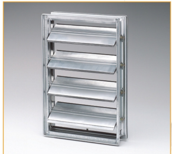
CD 60 — Galvanized Aerofoil Blades 152mm Max. air leakage — 0.07%, Min. size — 203x254mm Max. single section size — 1524x1829mm Max. multiple section size — Unlimited
