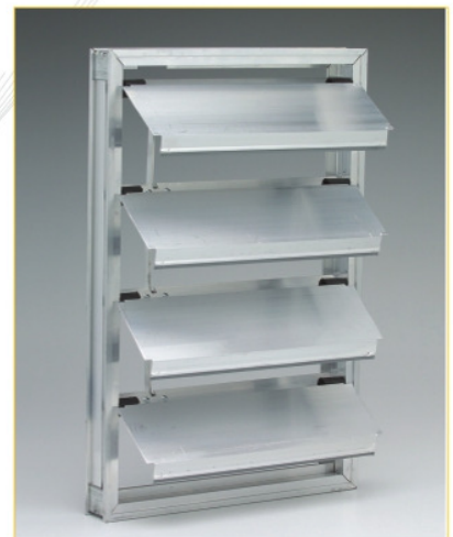
BD 6 — Extruded Aluminum Blades in 52mm frame, used for medium back draft duty conditions (30Pa-50Pa). Max. system velocity – 2500FPM Max. air leakage – 0.7% Min. size – 152x152mm Max. size single section – 1219x1321mm Max. multiple section size – Unlimited
