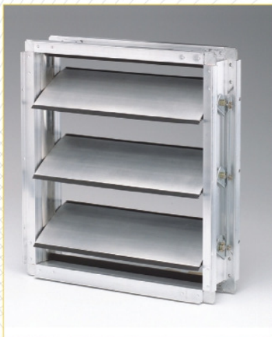
CD 50 — Extruded Aluminum Aerofoil Blades 152mm Max. air leakage – 0.07% Min. size – 152x229mm with opposed blade and 152x127mm with parallel blade Max. single section size – 1524x1829mm Max. multiple section size – Unlimited
