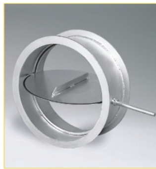
CDR 82 — All Heavy Duty Steel Construction Damper to control air flow within round ductwork in medium pressure industrial HVSC Systems. Max. air leakage – 0.32% with seal and 1.06% without seal Min. size – 102mm dia. Max size – 1524mm dia.
