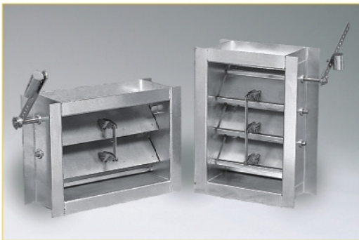
CBS 7 — All Galvanized Steel construction to meet industrial heavy duty requirements in 203X51mm frame. Max. system velocity – 3000FPM Max. air leakage – 0.67% with seals and 3.33% without seals Min. size – 152x152mm Max. size – 1219x2448mm
