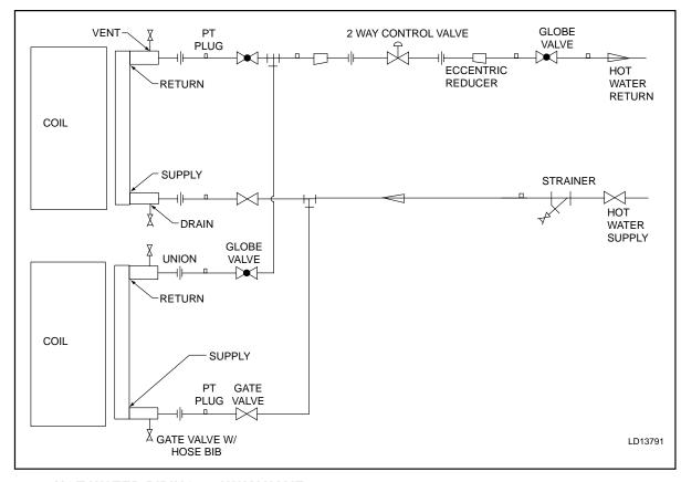
FIG. 2-69 - HOT WATER PIPING - 2 WAY VALVE
