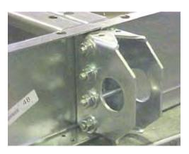
Baserail Lifting Lugs Assembled
