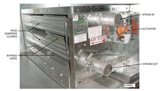
FIG. 2-72 - INTEGRAL FACE AND BYPASS COIL (HORIZONTAL; TUBES, STEAM SHOWN)
