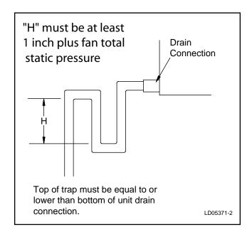
FIG. 2-92 – TRAP DETAIL FOR BLOW THROUGH APPLICATION
