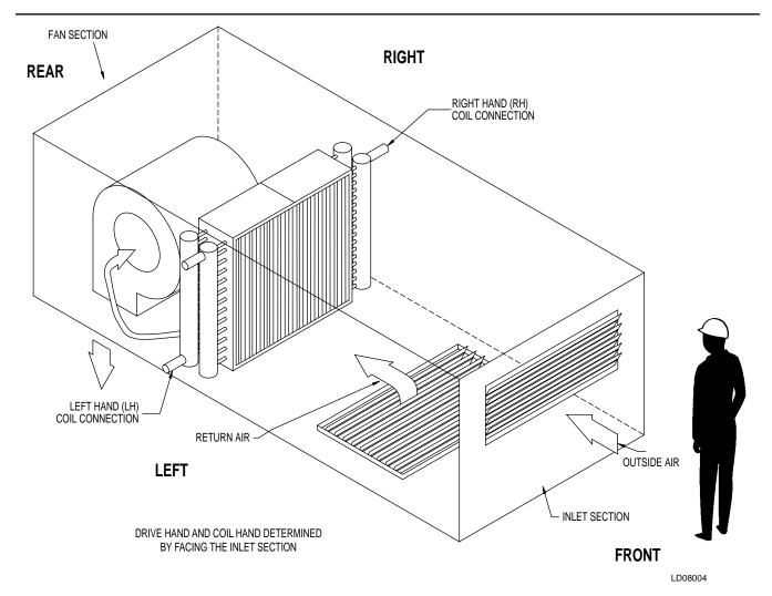
FIG. 2 – UNIT AND COIL HAND IDENTIFICATION
