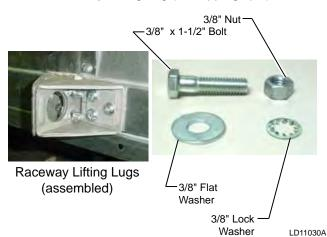
FIG. 2-9 – BOTTOM RACEWAY SHIPPING SPLIT FASTENER PACK P/N 386-03418-000 (4 each per pack)
