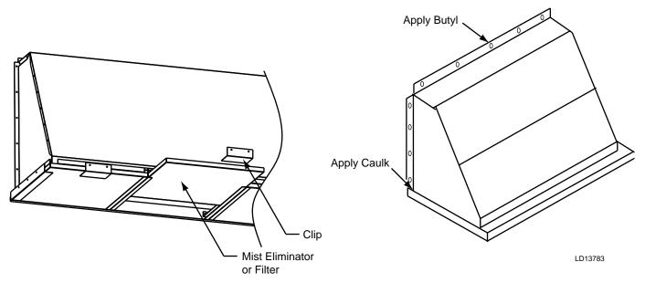
FIG. 2-34 - HOOD INSTALLATION WITH OPTIONAL MIST ELIMINATORS
