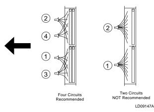
FIG. 2-83 – STACKED COIL CIRCUITING
