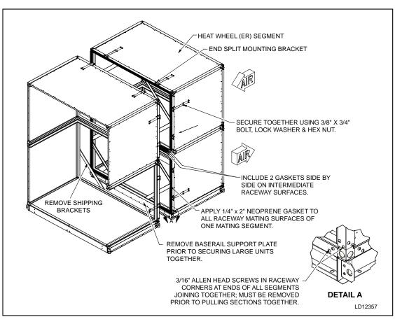
FIG. 2-33 – ASSEMBLY OF END CHANNEL SHIPPING SPLIT (ENERGY RECOVERY WHEEL SHOWN)
