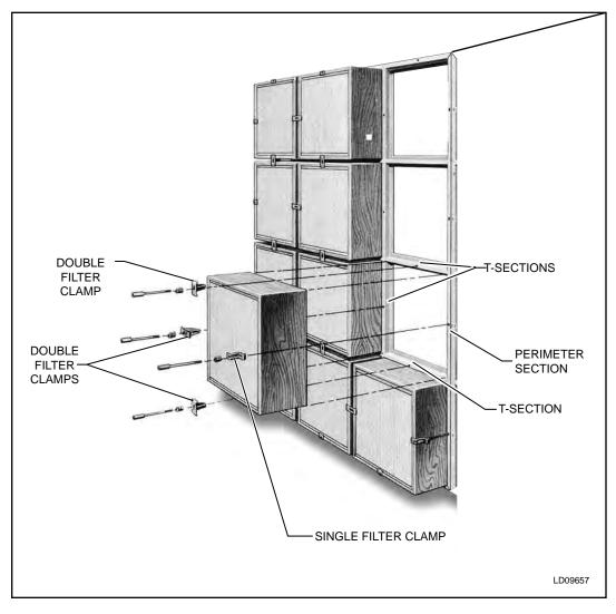
FIG. 2-118 - HEPA FILTER INSTALLATION
