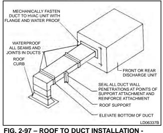
FIG. 2-97 – ROOF TO DUCT INSTALLATION -HORIZONTAL DISCHARGE
