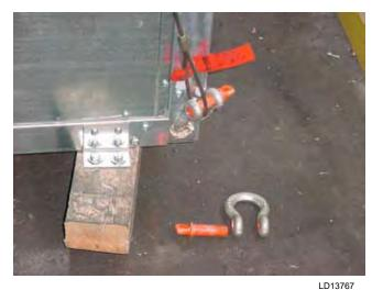
FIG. 1-4 – PROPER LIFTING WITH SHACKLE AT CORNER
