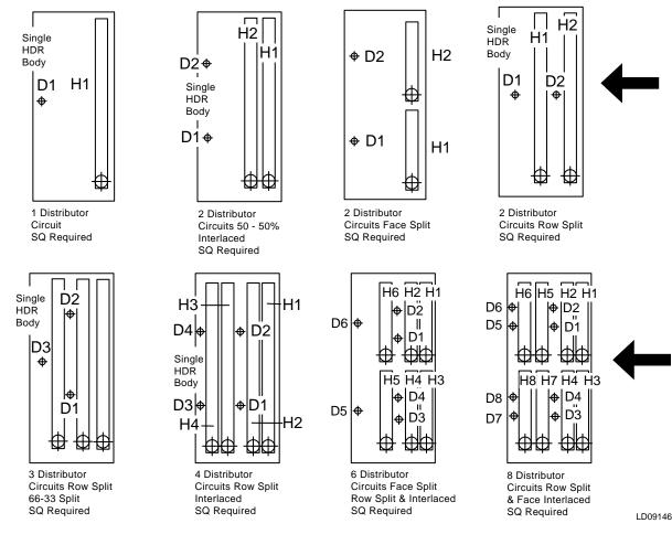
FIG. 2-82 – STACKED COIL DESIGNS - SQ SPECIAL JOHNSON CONTROLS
