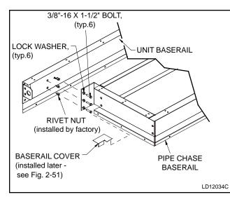
FIG. 2-43 – PIPE CHASE BASERAIL TO UNIT BASERAIL INSTALLATION (When Purchased)
