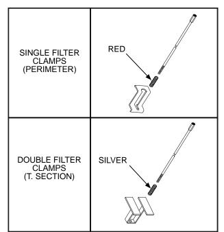
Used to attach HEPA Filters to Holding Frame.
