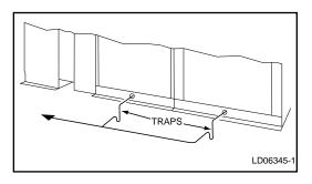
FIG. 2-93 – COMBINING DRAIN LINES
