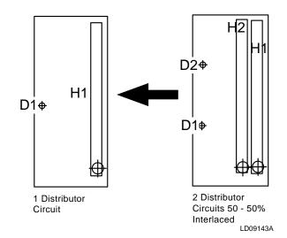
FIG. 2-80 – NON-STACKED COIL DESIGN -STANDARD
