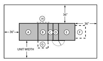
FIG. 2-1 – MINIMUM SERVICE CLEARANCES
