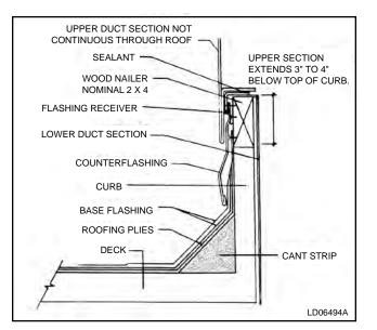
FIG. 2-96 - DUCT PENETRATION OF ROOF
