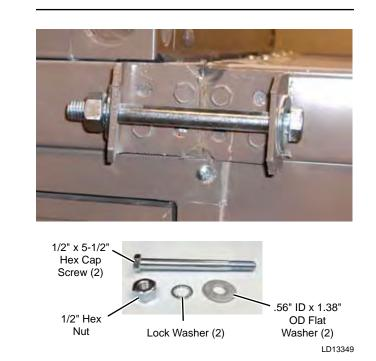
FIG. 2-11 – TOP RACEWAY SPLIT FASTENER PACK P/N 386-04747-000 (2 each per pack)
