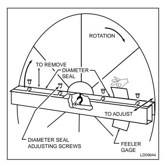
FIG. 3-13 - DIAMETER SEAL ADJUSTMENT
