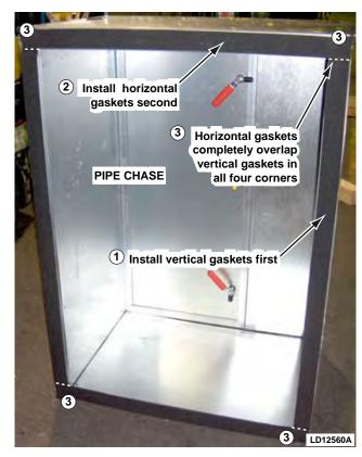
FIG. 2-42 – APPLY GASKET TO PIPE CHASE
