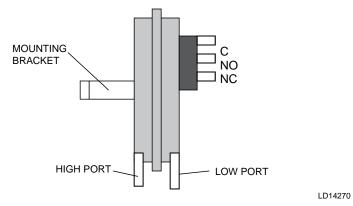
FIG. 3-27 – AIRFLOW SWITCH CONNECTIONS
