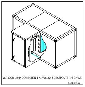
Usable working clearance is approximately the depth of the pipe chase minus 5".
