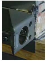
Raceway Lifting Lug (at shipping split)
