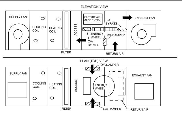
FIG. 3-10 - OUTDOOR UNIT - HORIZONTAL WHEEL
