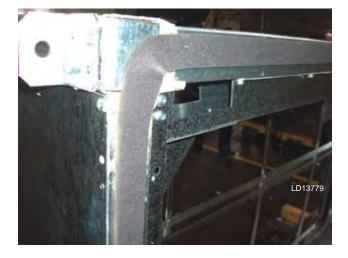
FIG. 2-21 – APPLYING GASKET TO SHIPPING SPLIT
