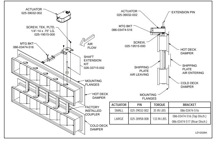
FIG. 2-36 – MZ DAMPER/ACTUATOR ASSEMBLY
