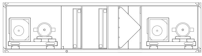
FIG. 1 – CUTAWAY OF YORK SOLUTION SHOWING VARIOUS SEGMENTS
