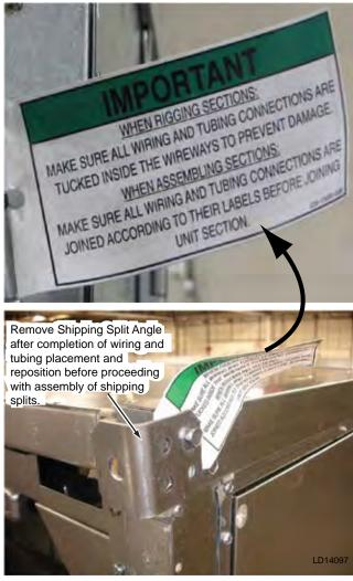
FIG. 2-19 – REMOVE AND REPOSITION SHIPPING SPLIT ANGLE
