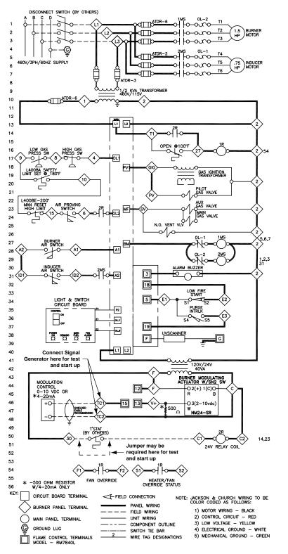
FIG. 3-24 – TYPICAL WIRING DIAGRAM
