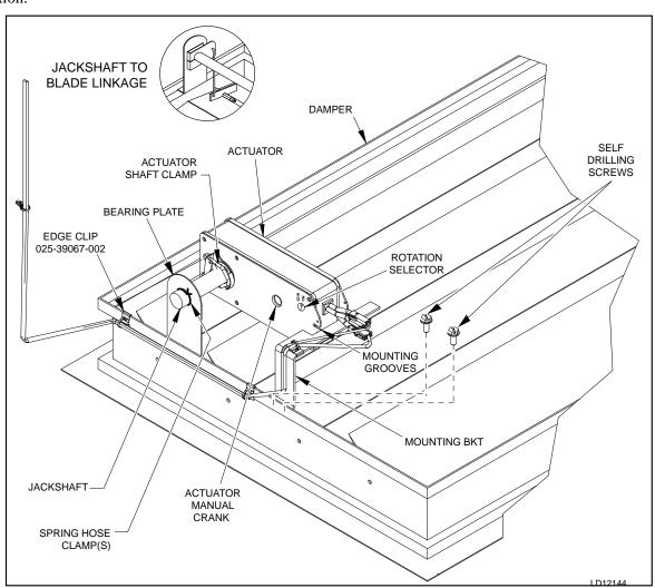
FIG. 2-35 – DIRECT COUPLED ON JACKSHAFT
