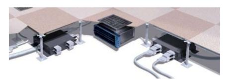
Control and power wiring are located under the floor, so they can be connected to the terminals via color coordinated plug-and-play connectors. Terminals can be added or removed to meet changing space configurations and loads, and control zones can be added or rearranged along with the furniture.
