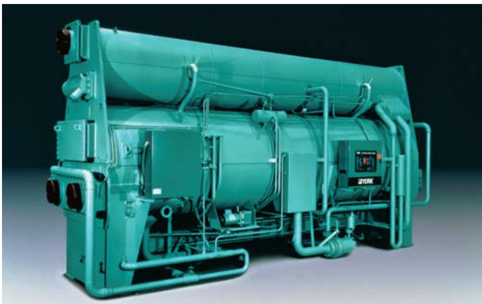
IsoFlow™ single-stage design for hot water or low-pressure steam. Units can use low-pressure steam (up to 1 bar or 15 psig) or hot water up to 130°C or 266°F for cooling in an almost unlimited number of applications.
