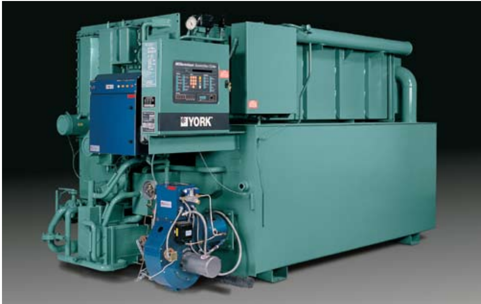
ParaFlow™ two-stage design for gas firing or high-pressure steam. Units can be driven by gas directly, or by high-pressure steam (2.8 to 8.8 bar or 40 to 128 psig). They can also output up to 82°C or 180°F hot water to serve as a high-temperature water heater.
