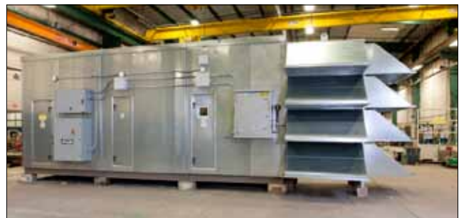
Figure 26 - Fresh Air Intake Plenum and Hoods Preassembled in the Factory
