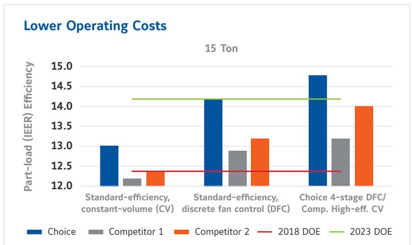
Standard-efficiency Choice rooftop units with the optional 4-stage IntelliSpeed™ fan control have better efficiency than even the "high-efficiency" models from competitors.
