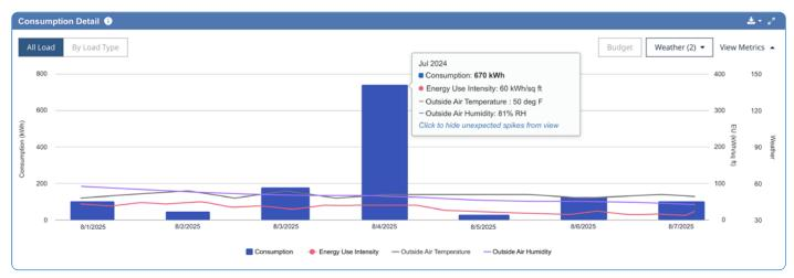
Report reflects a sudden spike in energy consumption, despite stable ambient conditions as indicated by the overlaid weather data. This suggests a possible equipment fault.
