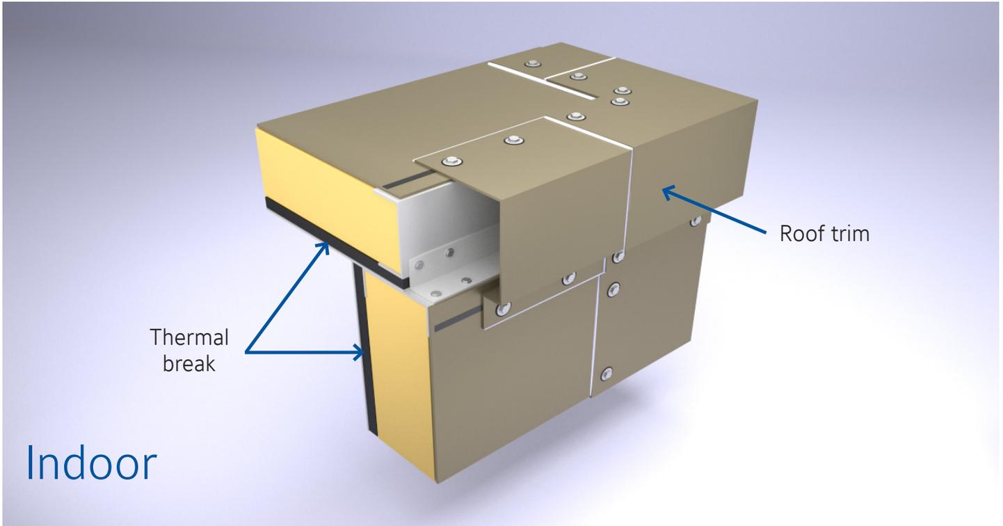
Roof panels are constructed using same materials and insulation as casing panels
