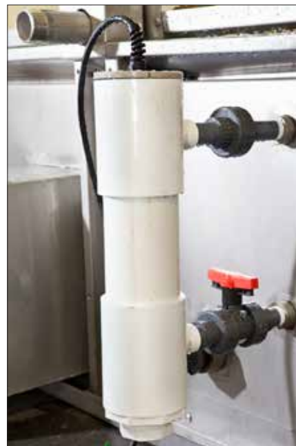
Figure 9 - Electronic Water Level Controller
