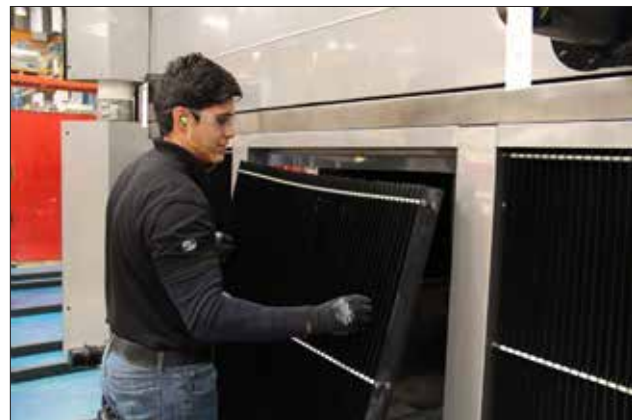
Figure 4 - Inlet Air Louvers
