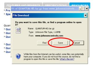
Select *Save* and save the update file to a Top Level root directory only. Saving to a subfolder will not allow the Quantum HD to recognize the file when the USB device is plugged in to the USB port of the Q5 processor board.
